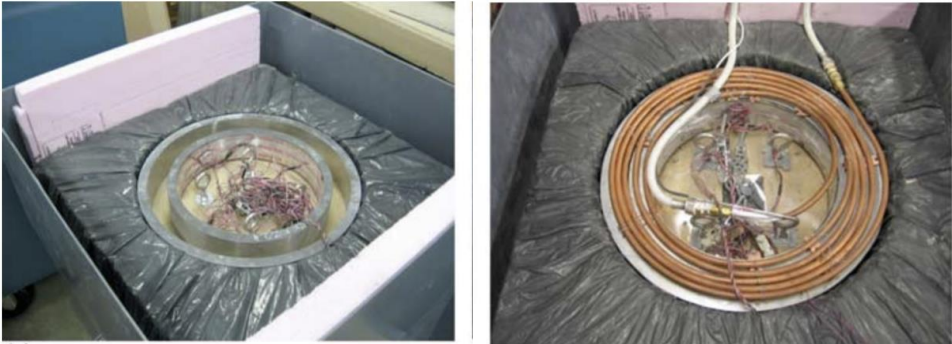
Figure 2: Examples of double-ring shrinkage test method [4].
