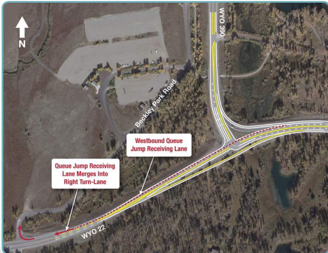
Figure 18: Concept 2, Westbound Queue Jump with Receiving Lane
