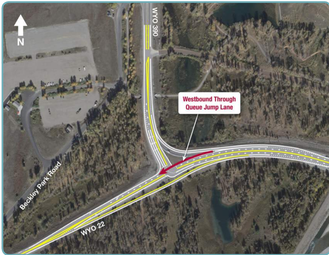
Figure 18: Concept 2, Westbound Queue Jump with Receiving Lane
