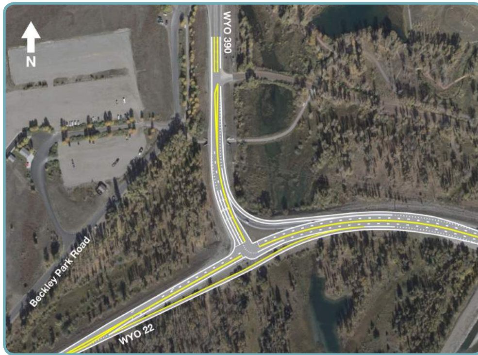
Figure 12: Proposed WYO 22/WYO 390 Intersection Improvements
