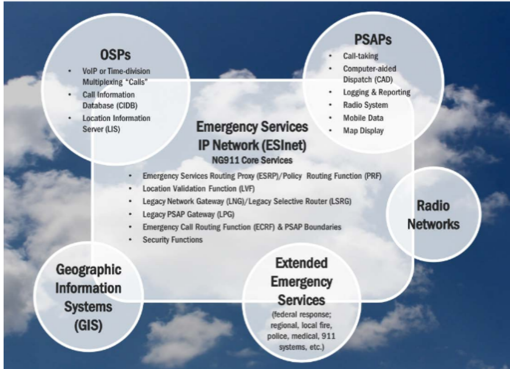
Figure 4 – NG9-1-1 System Components
